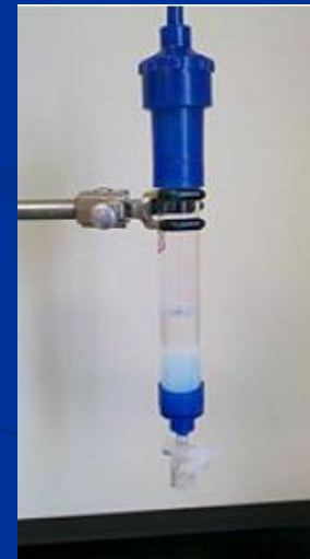
A chromatography column containing nickel-agarose beads used for purification of proteins with histidine tags
